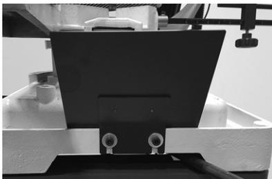
**Figure 18 - Front splash plate.**
