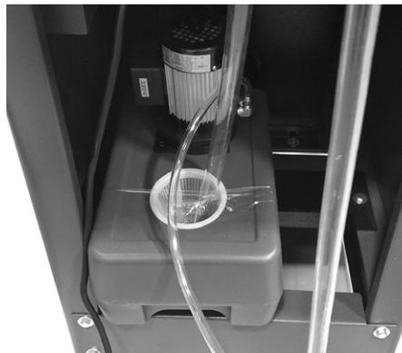
**Figure 17 - Install coolant tank.**
