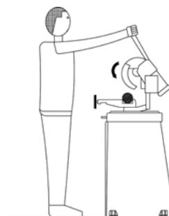
**Figure 26 - Operator position.**
