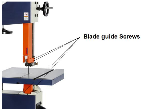
Figure 2: Blade guide screws
