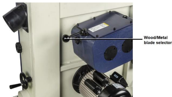
Figure 4: Wood/Metal selector switch
