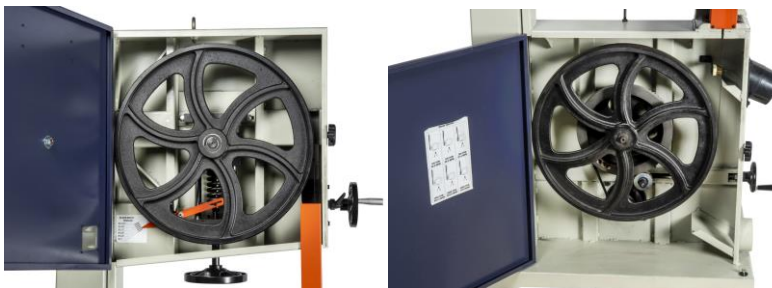
Figure 1, Open cabinets, top(left) and bottom (right)
