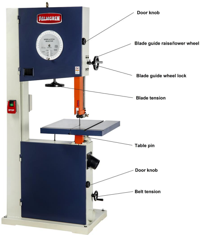
Figure 7: Handwheels and knob descriptions
