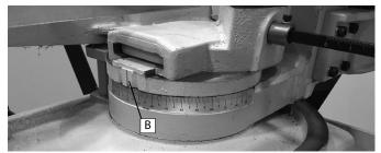
Figure 23 - Miter angle, angle indicator and angle gauge.
