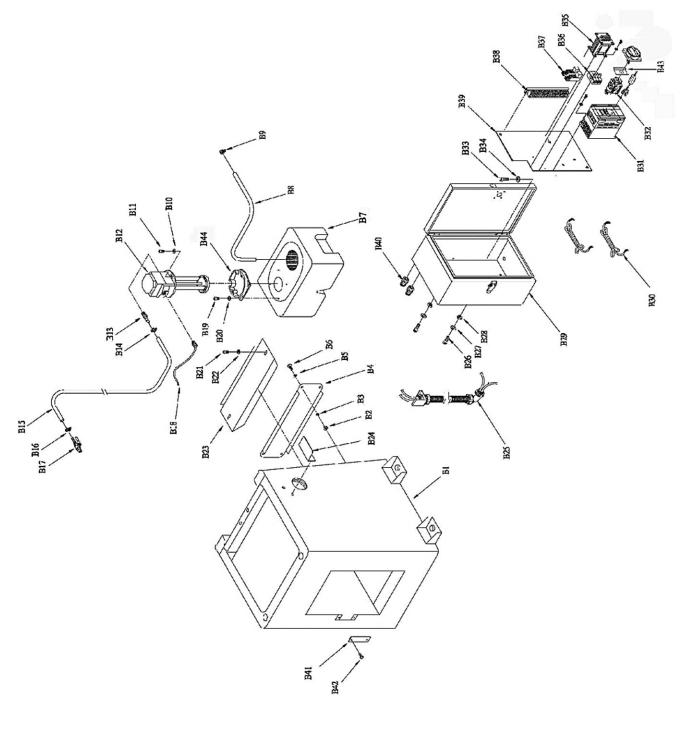
Figure 36 – Repair Parts Illustration for Stand.
