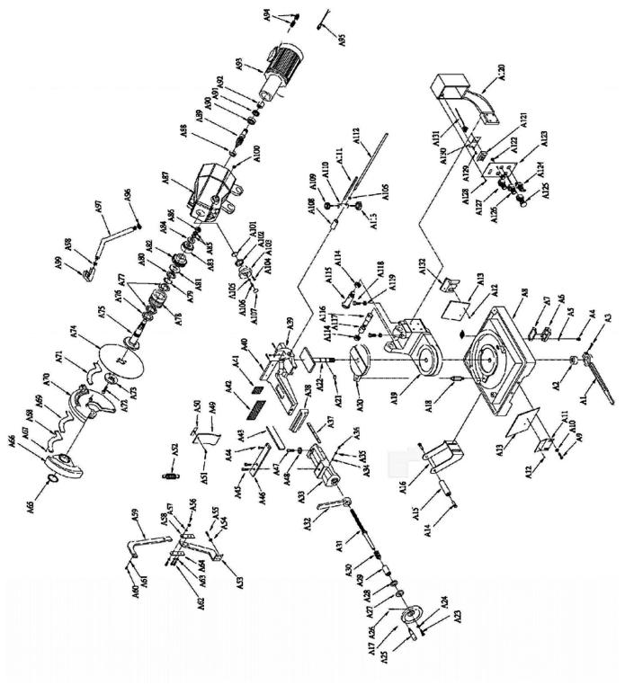
Figure 35 — Replacement Parts Illustration for 14" Variable Speed Cold Saw.
