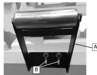
Figure 14 - Attach support roller to left side of base .
