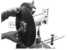
Figure 29 - Changing the saw blade.
