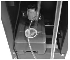
Figure 17 - Install coolant tank.
